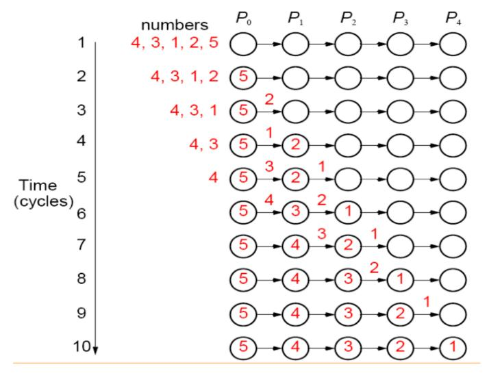
T<sub>pipelined</sub> = 2n, with n processors, so maximal speedup = n/4 - 3 ( wortcase sequential time = (n-1)(n-2)/2 )
