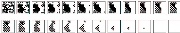
Fig. 2. This figure shows a correct classification of the Majority Problem by a two dimensional CA with both width and height equal to 13 and \lambda = 84/169 . The transition rule was one of the best tested in the experiment and scored F_{169,10^3} = 0.715 .
