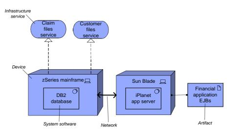
Figure 9. Example of a technology-layer model
