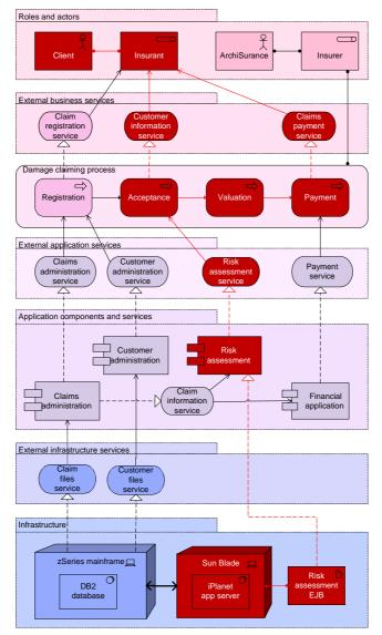
Figure 13. Example of impact analysis; darkened concepts show what is affected by failure of the Sun Blade server
