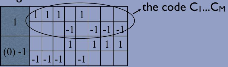
Now, each bit to be transmitted is encoded by: For  $I \le m \le M$ :  $Z_{i,m} = d_i c_m$
