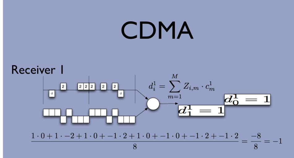
Receiver 2 is similar, but then code  $c^2$  is used. So, the trick is to find the right code so that this works!!!
