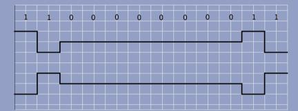
B8ZS (bipolar 8-zero substitution): Substitute eight '0' with:
