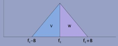
V≡W, so all frequencies between f<sub>c</sub>-B and f<sub>c</sub> can be filtered away.
