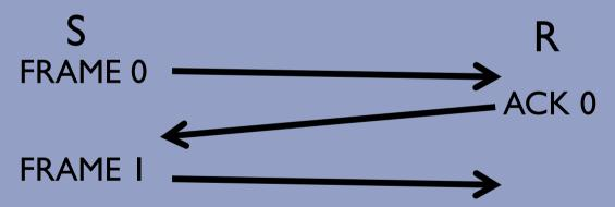
Transmission time per frame: t + 2a instead of t + a So if a (latency) is comparable to t (frame processing time), then 30% efficiency loss !!!!!!
