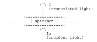
Light is absorbed progressively as it passes through a partly absorbent substance, if a single thickness reduces light intensity to half its original value, a double thickness will not absorb all light, but will reduce it to 25 percent.
