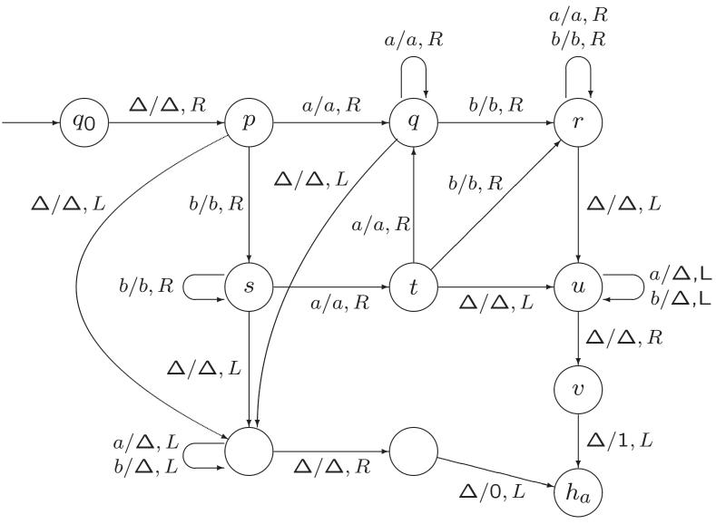
$q_0 \triangle aaba \vdash \triangle paaba \vdash \triangle aqaba \vdash \triangle aaqba \vdash \triangle aabra \vdash \triangle aabar \triangle \vdash \triangle aabua \vdash \triangle aaub \vdash \triangle aua \vdash \triangle ua \vdash u \triangle \vdash \triangle v \triangle \vdash h_a \triangle 1$
