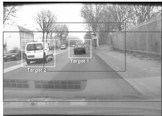
Figure 2: LSOD applied on real data. The vehicles in front of the camera are detected and tracked. The dark rectangles depict the area of the image that is processed.
